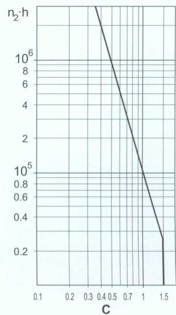
Radial loads on input shafts
