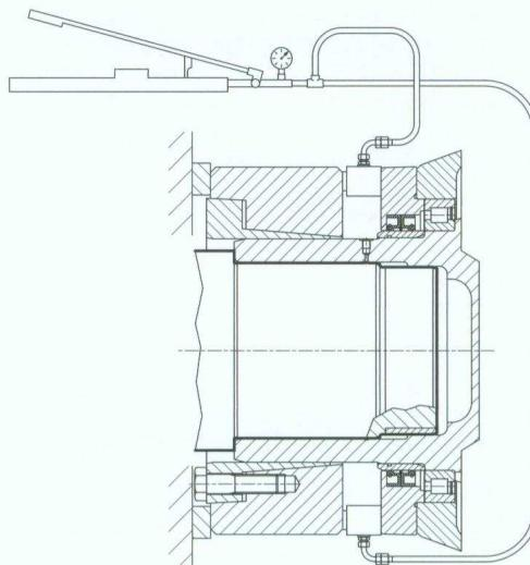
1) Loosen the screws in repeated sequence until the joint can be moved on the hub.
