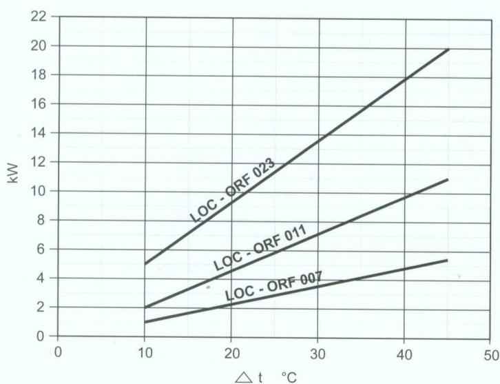
$$\Delta t = (T_{oil\ IN} - T_{air\ IN})$$
