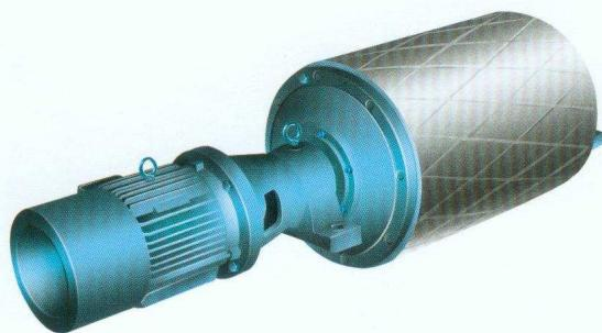
External Electric Roller is a new kind of Electric Roller, the motor is installed outside the body of roller, and the reducing mechanism is installed inside the body of Roller. It overcomes the shortcoming of poor radiating condition and limited working power, now the working power is up to 160kW and even bigger.
