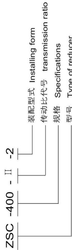
ZSC(D)立式大速比减速器 Vertical big transmission ratio of ZSC(D) decelerator
